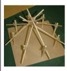
How could we strengthen the roof even further? Allow chn to suggest creating triangles with lolly-sticks going across each beam.
